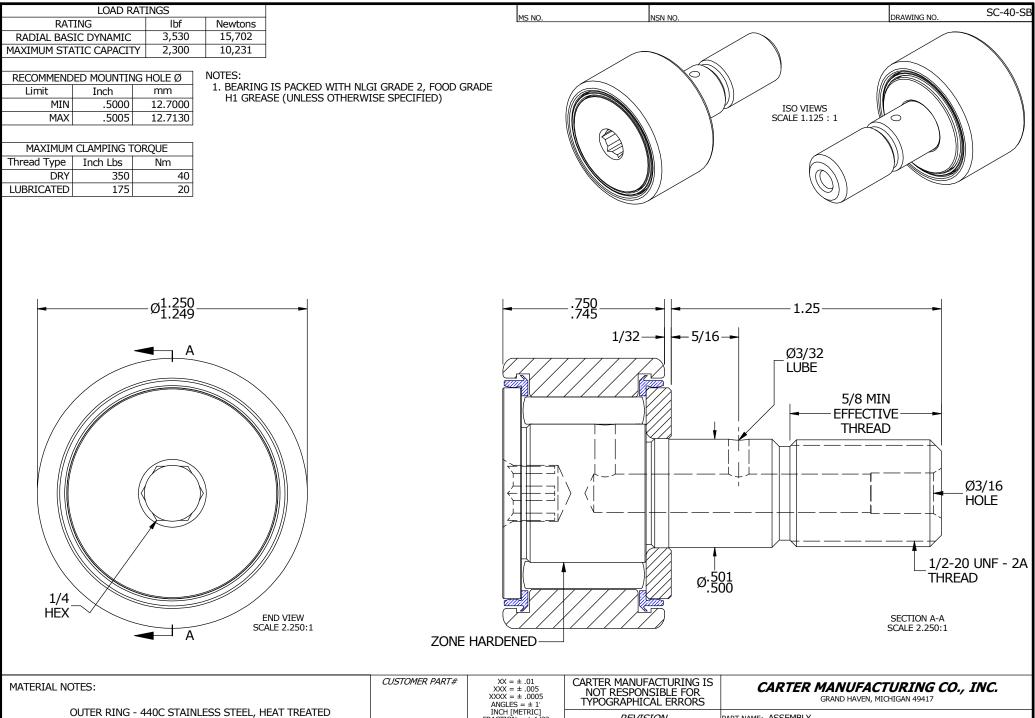
STUD - 440C STAINLESS STEEL, ZONE HARDENED NEEDLE ROLLER(S) - 440C STAINLESS STEEL, HEAT TREATED WASHER - 440C STAINLESS STEEL, HEAT TREATED SEAL(S) - SYNTHETIC
