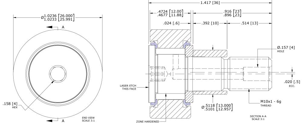
\*\*TORQUE SPECIFICATION IS BASED ON LUBRICATED THREADS, IF USING DRY THREADS DOUBLE TORQUE VALUE
