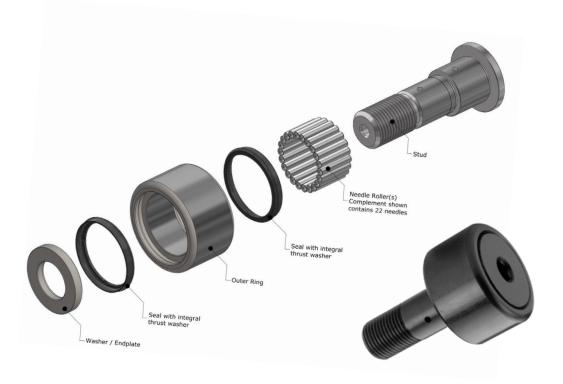
Stud-type cam followers include a partially threaded shaft fixed to the follower inner diameter (ID) for assembly onto a machine frame with a nut or similar fastening device.
